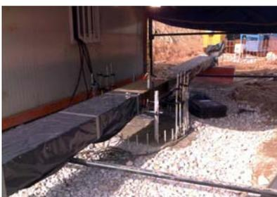
O-cell bi-directional testing setup
